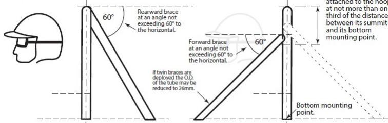
Fig. 2. Roll over protection structure bracing guidelines
